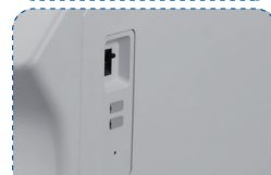
USB port for exporting operation record including speed, time and temperature, operation curve with alarm messages etc.
